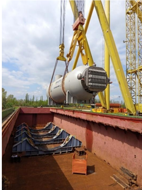
Figure 8: First manufactured second-generation pool condenser for the ULE Design ready for transport.
