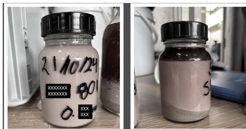
Figure 6: Urea and nutrient(s)-bearing solid well-dispersed in urea melt (L) and settled (R)
