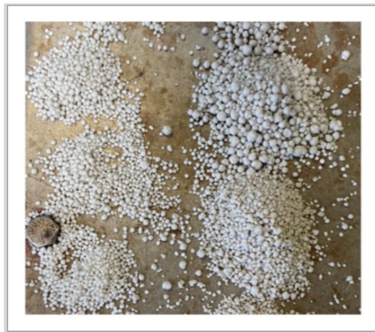
Figure 13: Slurry granulation particle growth over time.
