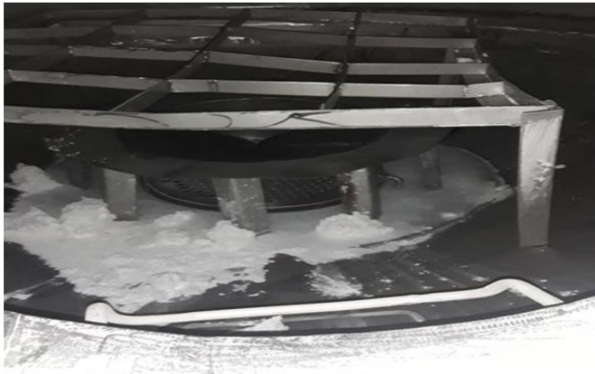
Figure 4 As found condition of S-402 after 1.5 years operation, with flushing practices
