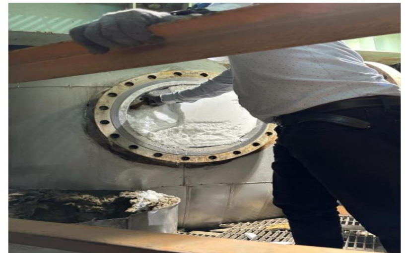
Figure 2: As found S-402 (heavily choked)
