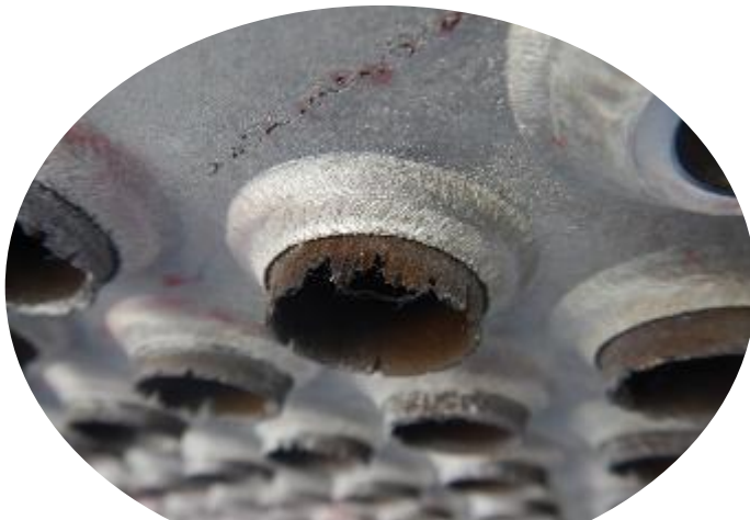
Severe cross-cut end attack
