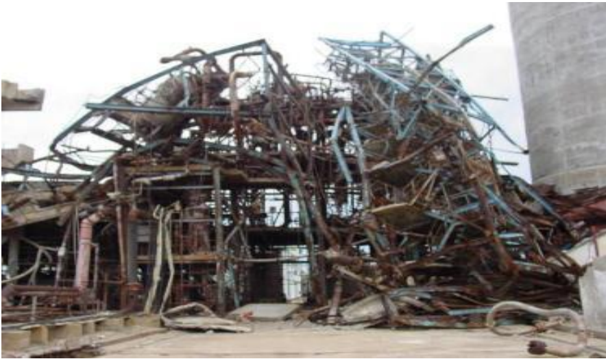
Catastrophic failed reactor of a 200 mtpd urea plant
