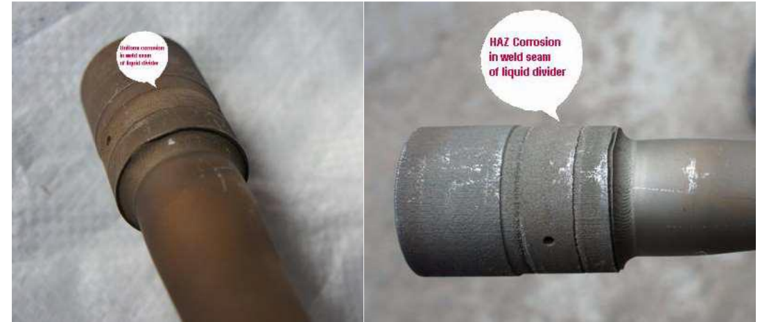
2012 : Weld seam corrosion / HAZ corrosion.
