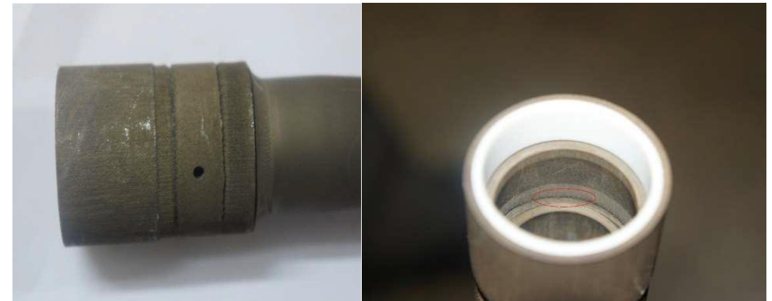
2014: Corrosion on external and internal weld seam
