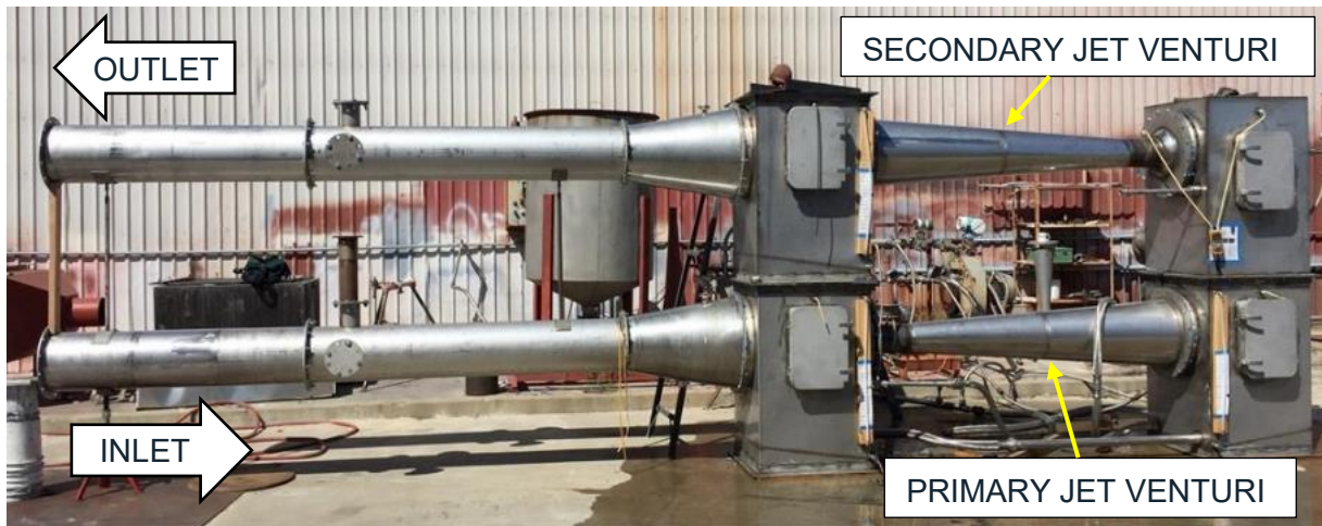
Figure 4: A two-stage Jet Venturi Scrubber pilot unit.
